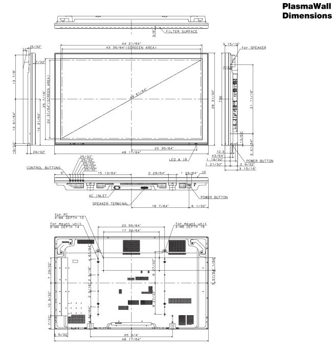
Figure 7-1 and Figure 7-2 show the PlasmaWall dimensions (all dimensions are in inches).
